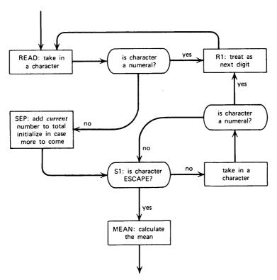
FIGURE 2.4 Flow chart to accompany the program in Figure 2.3.
