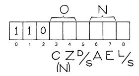
Since bits 0 and 1 are set to 1, and bit 2 to 0, the 9-bit instruction code for Test instructions is always between O 600 and O 677. All sixty four combinations give valid instructions. The mnemonics are three or four letter codes, of which the first is T. The second letter is R (right), L (left), D (direct) or S (swapped).
