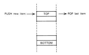
The subject of pushdown lists is by no means as obscure as might appear on first impressions. Successive quotients in a printout routine, and the start addresses of successive nested subroutines, are two of the many examples of information that is handled on just such a "last in, first out" basis.
