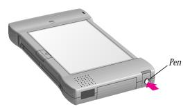
Push and release the end of the pen to take it out. You can also pull out the pen holder, just above the pen compartment, to hold your pen when it's not in use.
