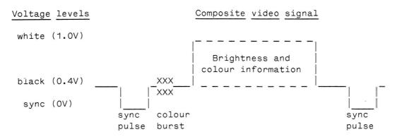
The sync pulses shown are for horizontal syncronization, and occur at 64us intervals. There are additionally vertical sync pulses which occur for about 0.5ms every 20ms.
