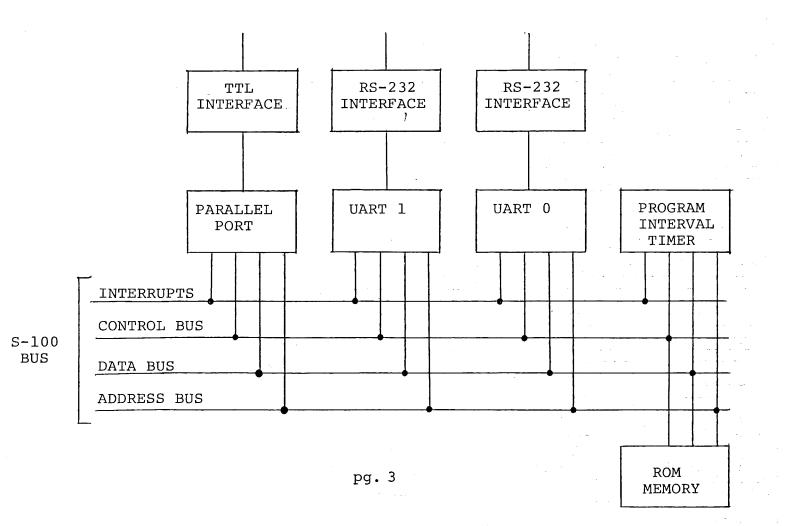
FIGURE 1 - Z80 CPU BLOCK DIAGRAM
