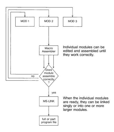
Figure 1. The Assembly Process
