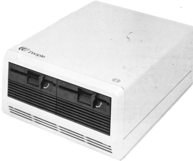
All of the electronics in the basic system are contained on two printed circuit boards. It uses the INTEL 8086 Microprocessor.
